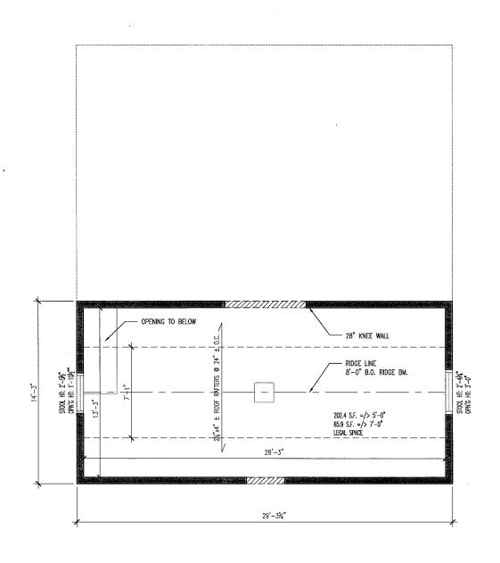
EXISTING/DEMO SECOND FLOOR PLAN SCALE: 1/4" = 1'-0"
